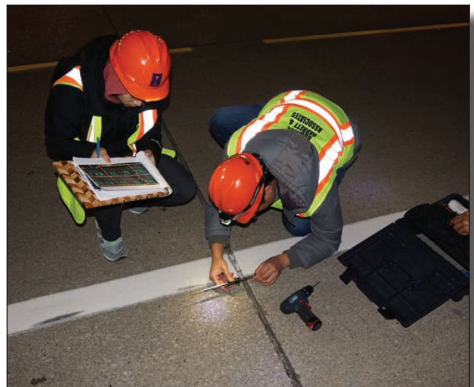
Figure 4. Students manually record displacements across joints
